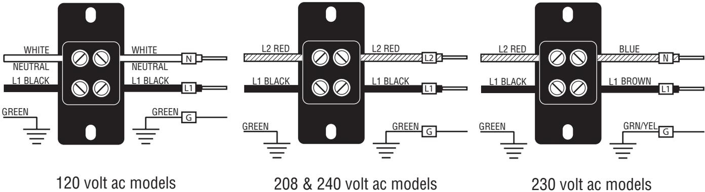
Note: This electrical service consists of 2 current carrying conductors (L1 and Neutral) and a separate conductor for earth ground.
