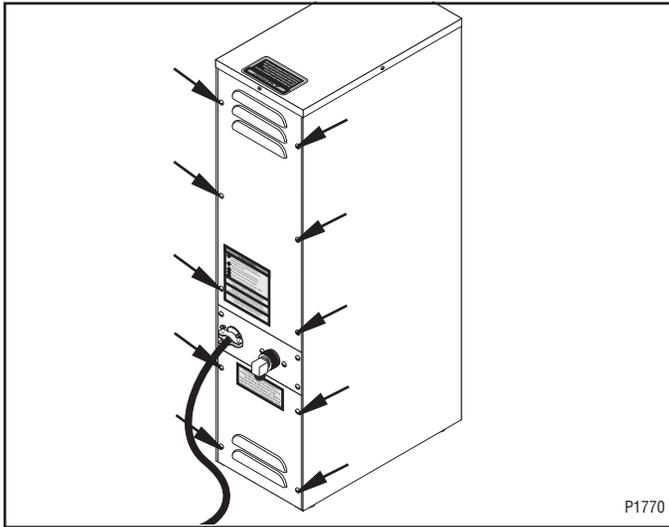
The check valve, electronic control board, safety overflow switch, solenoid valve, overflow tube temperature sensor and terminal block are located at the rear of the dispenser. Access is gained by removing the upper and lower rear panels. The upper is attached with six 8-32 slotted-head screws. The lower is attached with four 8-32 slotted-head screws. The middle panel must not be removed from the dispenser.
