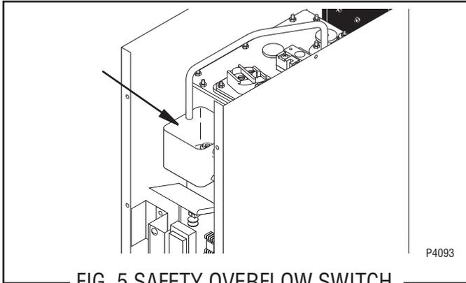
FIG. 5 SAFETY OVERFLOW SWITCH
