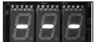
3. When the factory default numbers are loaded in, the display will stop flashing, then read **don** (DONE). You can now release the two buttons.
