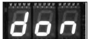
**NOTE:** If you release the two buttons at any time before the display reads **don**, the Factory Default numbers will not be entered. The old numbers will remain in the memory.
